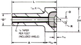
MoldStar®150 material (Beryllium free) body, with hardened 420 S.S. insert at nozzle seat area, Carbide-lined sprue channel
